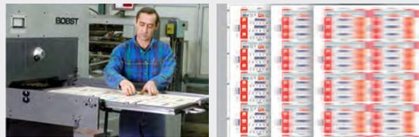
None of that! Now is the time for optimized and industrialized cutting techniques. At first cut of a new job the operator can adjust the cutting pressure up to 90% in the cutting area. Only the remaining 10% in the non-cutting area have to be patched accordingly.
